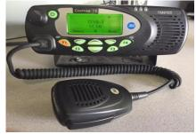
operations to maintain contact with the deployed teams. For simplex operations in the mountains, it may provide you a better option for reaching search teams. Be careful the squelch is not set too tight on this radio as it will severely impact your ability to hear weak signals during simplex operations. New photos will be provided at that time.
