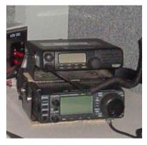
The HF rig is an ICOM IC-706 IIG (under the FT 2600). A remote antenna tuner is mounted in the storage cabinet and controlled from the front of the IC-706. This set can be used for HF Amateur or MARS operations. A set of Hamstick HF antennas are stored in the Antenna Cabinet to the right of the main van entrance and accessible only from outside the truck. Select the one you need for the
