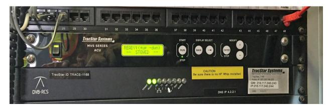
To shut down the satcomm, press the "RUN" button until the "STOP" LED is on. Then press and the "-" key on the right side of the panel for 2 seconds. The display should now indicate that the antenna is "Stowing". When the Antenna warning lights stop flashing on the main control panel and the dash board, you will know that the antenna is in the "stowed" position.
