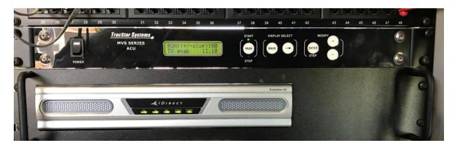
To shut down the satcomm, press the "**RUN**" button until the "**STOP**" LED is on. Then press and the "-" key on the right side of the panel for 2 seconds. The display should now indicate that the antenna is "Stowing". When the Antenna warning lights stop flashing on the main control panel and the vehicle dash board, you will know that the antenna is in the "stowed" position.
