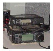
The HF rig is an ICOM IC-706 IIG (under the FT 2600). A remote antenna tuner is mounted in the storage cabinet and controlled from the front of the IC-706. This set can be used for HF Amateur or MARS operations. A set of Hamstick HF antennas are stored in the Antenna Cabinet to the right of the main van entrance and accessible only from outside the truck. Select the one you need for the
