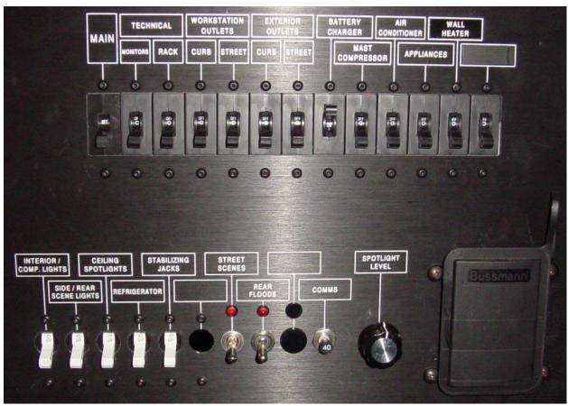
The top row switches are breakers for AC power and the bottom row are all DC power. Typically, all the AC power are turned on except the wall heater. The wall heater and
